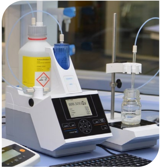
Figure 4: Xylem burette Titronic® 500, used for polyamide solution preparation. The burette is available with special dosing units suitable for corrosive and high-viscosity solvents such as concentrated sulfuric acid
