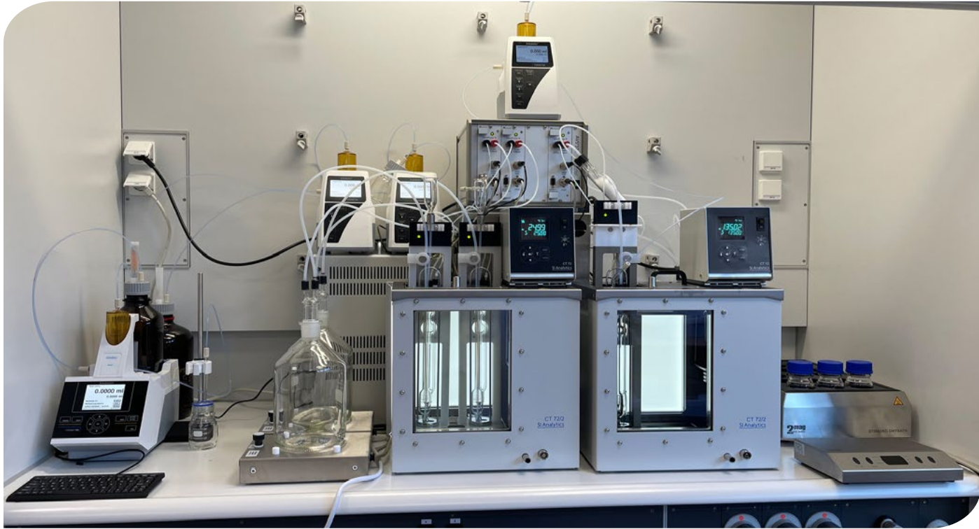
Figure 1: Viscometry measuring system AVS® 370, positioned in a fume hood at KraussMaffei Extrusion GmbH, Hannover. 1
